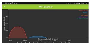
• The RF Spectrum Analyzer scans the 2.4GHz band for any Wi-Fi signals, and displays them in a graph by both strength and frequency.
