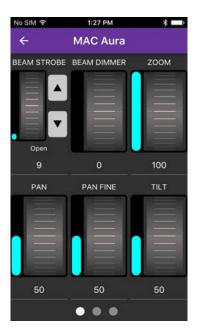
• After selecting the fixture, choose the starting DMX address of the fixture, and press "Next" and the fixture's user interface appears.
