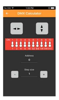
•Either type in a DMX value to read the corresponding to DIP switch, or vice versa.
