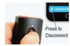
Press the "LINK" icon to disconnect the DMXcat. Press and hold the power button until the LED indicator flashes four times.
