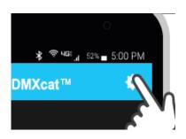
Press the "SETTINGS" menu on the upper status bar, and select "Device List" and select your DMXcat. <u>The SN to identify your DMXcat</u> <u>is located on the back of the device.</u>
