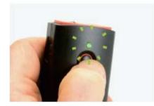
Turn on the device by pressing the power button- the LED status indicator will flash green.
